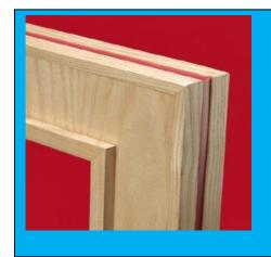
Intumescent strips fitted to the edges of the door – because there are no cold smoke seals it is permissible to paint over the intumescent strips with a maximum of five coats of conventional paint or lacquer or a maximum of 0.5 mm, whichever is the greater.
