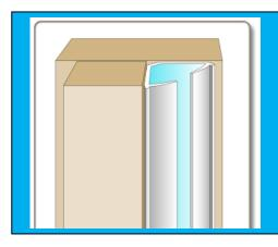
PVC, acoustic and cold smoke perimeter seal located in the corners of rebated frames of fire doors. Under no circumstances should this seal be painted
