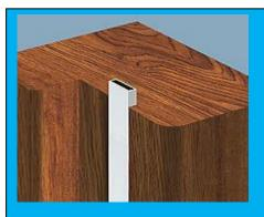
Intumescent strips fitted to the **door frame** – because there are no cold
